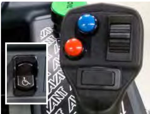
Hand drive controls enables the forward-reverse driving of the loader with a switch on the joystick, instead of the drive pedals. The hand drive is proportional like the drive pedals: the more the switch is turned the faster the machine will travel. It is possible to use either the hand drive or the standard drive pedals; selection between hand drive and pedal control happens with a switch on the dashboard.
