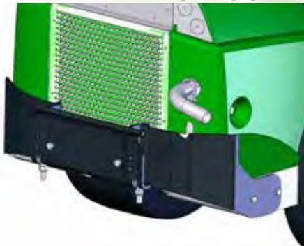
Makes it possible to mount and transport attachments in the rear. The standard 400 lbs rear bumper must be removed, and extra counterweights, rear side weights and trailer couplings can not be installed.
