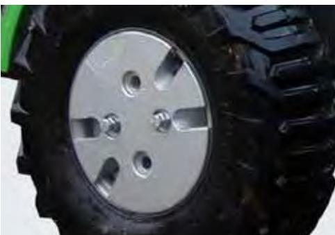
Avant 200 series can be equipped with 3 l lbs wheel weights which mount on the rim with special bolts. They make the center of gravity of the machine lower and add weight, which improves the stability of the loader.
