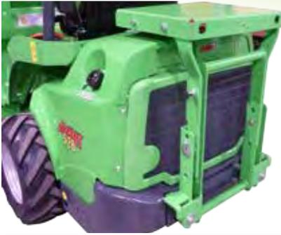
The tiltable rear carrier mounts on the rear bumper with bolts. It is standard equipment on rear mounted generator, compressor and pressure washer.
