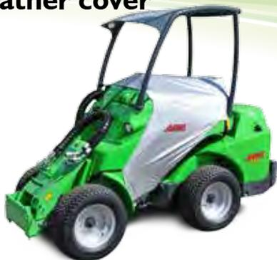
Weather cover protects the cockpit against rain, snow, dust and dirt. The weatherproof cloth covers the entire instrument panel, steering wheel and driver's seat. The weather cover is delivered with an integrated pouch where the cover can be wrapped when not in use.
