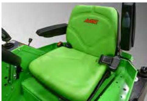
Suspension seat is optional equipment on 200 and 400 series. It is equipped with arm rests, seat belt and heater.
