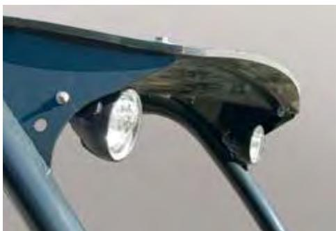
The work light kit consists of three LED lights: 2 to the front, 1 to the rear. Two types of LED lights available: 700 lumen or 2400 lumen.
