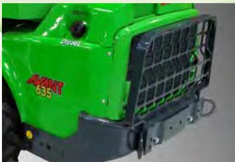
The rear guard protects the rear and the radiator of the engine. It mounts with four bolts and is easy to install and take off. The rear guard is equipped with tie down brackets and allows mounting of back weights and/or trailer coupling at the same time.
