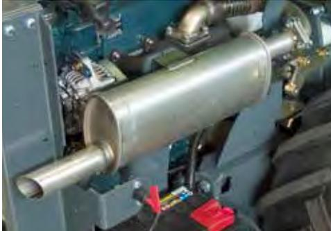
Exhaust purifier can be mounted instead of the standard exhaust muffler. It reduces diesel engine emissions.
