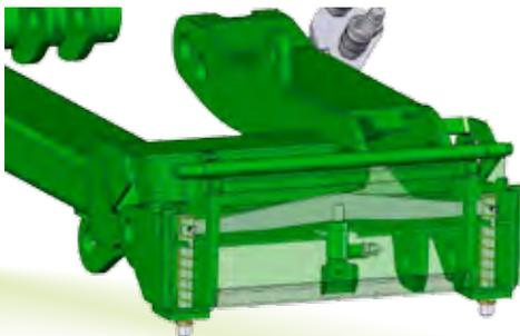
The hydraulic attachment coupling plate enables coupling and disconnecting of the attachment from driver's seat. There is a hydraulic cylinder on the attachment coupling plate which moves the locking pins up and down. The electro-hydraulic system works also when the engine is not running, as long as the ignition switch is in "ON" position (current on).
