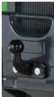
There are two types of trailer couplings available: a 2 inch ball hitch and a 2 inch ball hitch with towing pin. Both can be mounted either directly on the rear bumper or on the extra back weight. Avant 200 series is equipped with a 2 inch ball hitch as standard.
