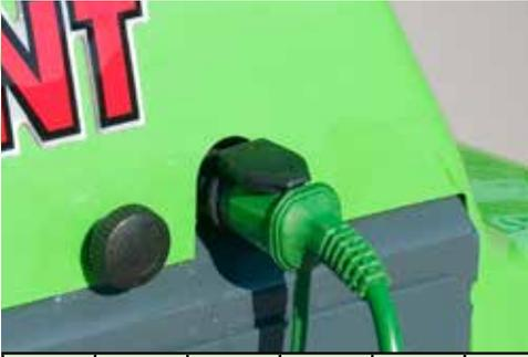
Engine heater facilitates starting in low ambient temperatures and saves the engine and reduces fuel consumption when starting in the cold.
