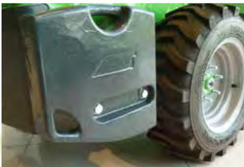
Rear side weights mount behind the rear wheels. They are delivered in pair: one on the left and one on the right side. Weight of the kit is 176 lbs, and it is intended mainly for 400 series, but can be mounted on bigger Avants as well.
