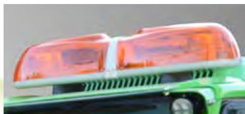
The beacon light bar is available for cab DLX only, instead of the rotating warning beacon.
