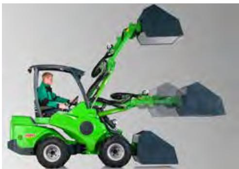
Self levelling system keeps the position of the attachment the same in relation to the ground, regardless of the position of the boom. Self levelling is hydraulic: there is a levelling cylinder on the left side of the boom which follows the movements of the bucket tilt cylinder and keeps the attachment level. Self levelling is disabled when boom floating is switched on. Avant 200 series is equipped with a self levelling boom as standard. The self levelling system is mechanical.
