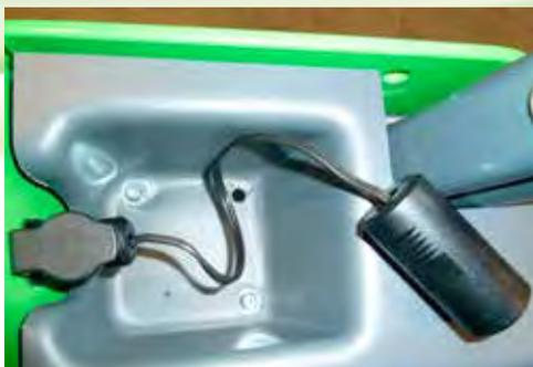
Connection cable, mounts on the 12V outlet on 400-800 series and 200 series I. Equipped with a connector where you can connect a cigarette lighter plug, for instance when using a mobile phone charger.
