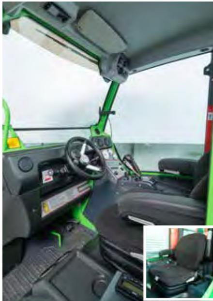
The top of the range cab DLX is equipped with heater, noise reducing interior materials, radio, cab air filter, LED work light kit, road traffic light kit, front and rear mudguards. Air conditioning, air suspension seat and beacon light bar are available as an option. A/C unit can be mounted either on the roof - or behind the rear window if a lower machine height is required. The spacious and ergonomic cab DLX represents modern cab design at its best.
