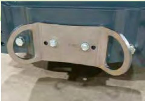
The bracket can be mounted on rear bumper and/or behind the rear wheels. Makes it easier to tie down the loader on a trailer etc.
