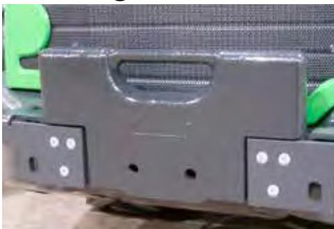
The extra 64 lbs counterweight mounts on the rear bumper. It is equipped with handle and fastening hooks, so it is easy to just drop the weight on the bumper, and also to drop the weights on each other. Trailer couplings A417323 and A417337 can also be mounted on the weight.
