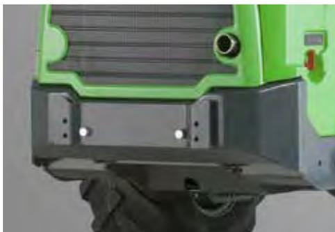
Avant 500 and 600 series are equipped with the 400 lbs rear bumper as standard, but if a lighter machine is required – for instance when driving on surfaces with limited carrying capacity – the light rear bumper can be installed instead of the standard bumper. It reduces total machine weight by about 330 lbs.
