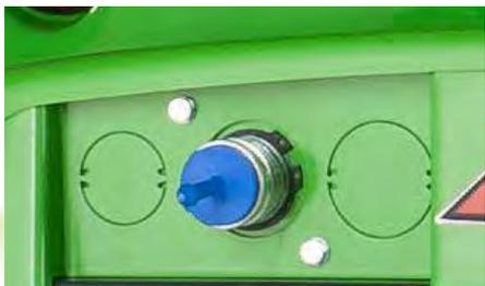
Single acting rear auxiliary hydraulics is equipped with one pressure line. It makes it possible to operate hydraulic attachments with single function.
