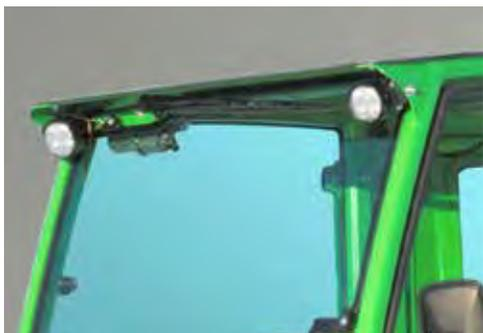
The work light kit can also be mounted on cab LX, with the same 700 lumen or 2400 lumen lights.
