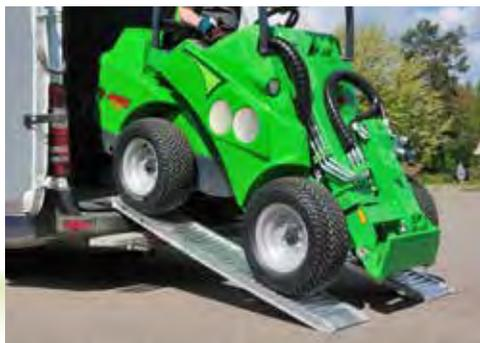
The lightweight and durable aluminium ramps are easy to handle and they stay clean thanks to the open grid design. Max. load is 4960 lb.
