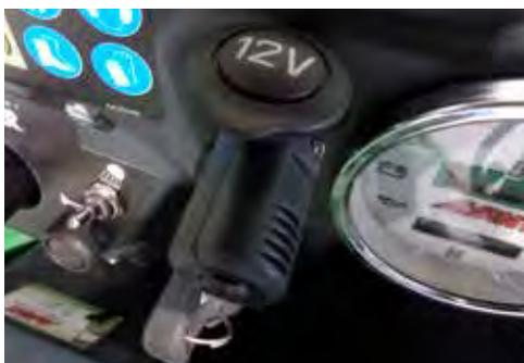
Adapter plug to 12V outlet, mounts both on the smaller 12V outlet on 400-800 series and on the bigger outlet on 200 series. You can connect the electric wires of any 12V electric appliance (for instance a battery charger) to this adapter. Requires therefore some electrician skills.
