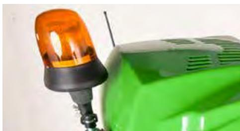
The rotating warning beacon is equipped with a very bright xenon lamp. It mounts on a tiltable socket and is easy to install and take off.
