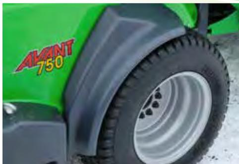
Rear mudguards are available as an option on a new machine, they cannot be retrofitted.
