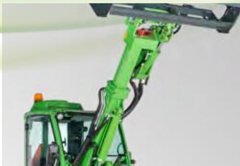
Telescopic boom gives more outreach and lifting height, which helps loading and reaching a lot. It is also easy to adjust the distance between the front wheels and the attachment with the telescopic boom, and you can also push the loader with the teleboom if necessary. Depending on model, telescopic boom gives 15.7-27.6 in more outreach, and the extra lifting height is about 15.7 in.
