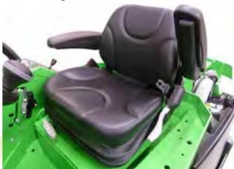
The full suspension seat with larger suspension is standard equipment on 600, 700, and 800 series. It is equipped with seat belt, arm rests and heater.
