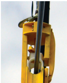
Cable Capture Prevents Pull Tape Or Cable Jumping Edge
