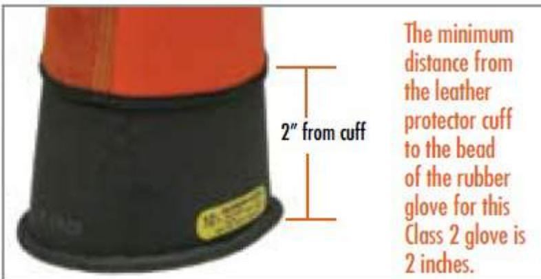
Leather Protectors are NOT to be used alone for electric shock protection. Always use gloves with appropriately insulated voltage ratings.
