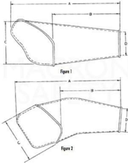
When choosing the proper sleeve size, they should fit comfortably, covering from the top of the shoulder to just inside the top of the glove. Select the shortest length possible while maintaining complete coverage to the shoulder.
