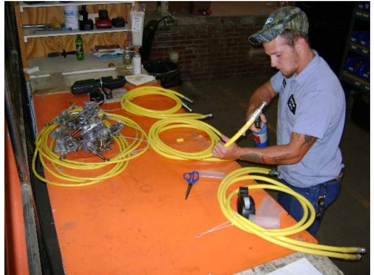
Special Fleet Service will custom build grounds and jumpers to your exact specifications. With a large quantity of parts in stock, we waste no time getting your equipment made and shipped to the field.
